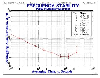
Figure 3. Stability of CSAC Physics w/Laboratory Electronics
