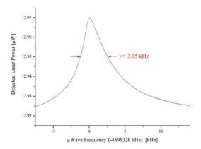
Figure 9. CPT "clock" resonance
