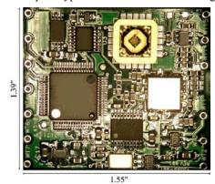
Figure 5. MAC Prototype PCB
