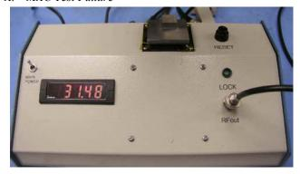
Figure 7. Prototype MAC Installed in test fixture
